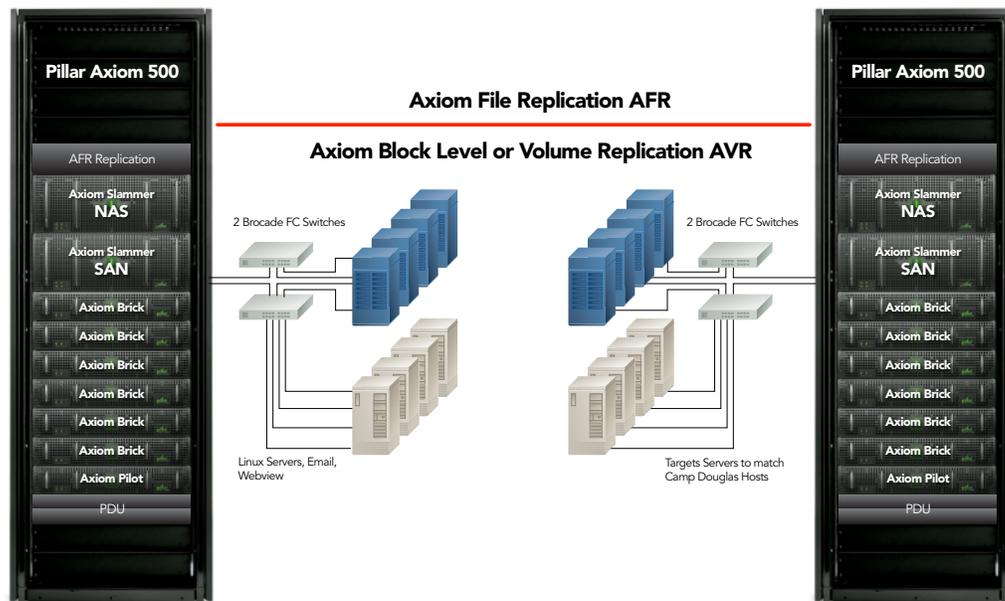
The deployment included two Pillar Axiom 500 storage systems, each with both SAN and NAS Slammers (four active storage processors and 12GB mirrored cache each), over 26TB of raw capacity per system, and dedicated switched FC backplane and redundant power distribution units. The system allows for end-to-end full redundancy, high-availability access to applications and data, and significant room to scale capacity while maintaining performance.
